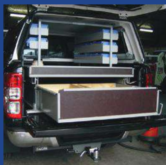
Ford Ranger Ute Roll out Large Draw, Roll out Adjustable Shelving facing outwards
