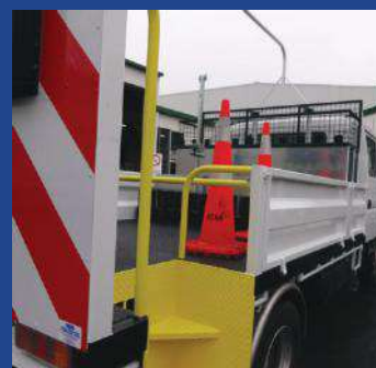
Truck COF Body Repairs & Modifications Towbar, Tie Rails, Load Hooks, Certified Welding
