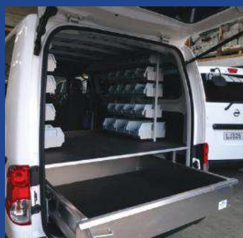
NV200 Van Single Alum drawer, False Floor, Adjustable Shelving
